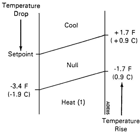
(1) If High Speed Heat Lockout is enabled, Heat is replaced by Null at setpoints below 15 F (-9.4 C)
