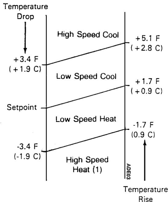
(1) If High Speed Heat Lockout is enabled, High Speed Heat is replaced by Low Speed Heat at setpoints below 15 F (-9.4 C)
