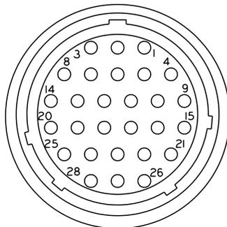
**Connector on Back of Single Temperature In-Cab TG-V**
