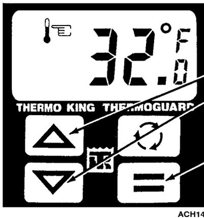
2. Press the UP or DOWN key until the setpoint is at exactly 32.0 F or 0.0 C.
