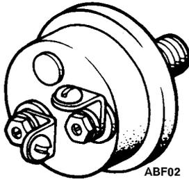
Engine Low Oil Pressure Switch
