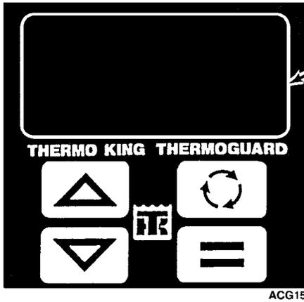
When the Thermo King unit is switched ON, all symbols and readouts will be displayed for about 5 seconds. Make sure that all display segments are operational.
