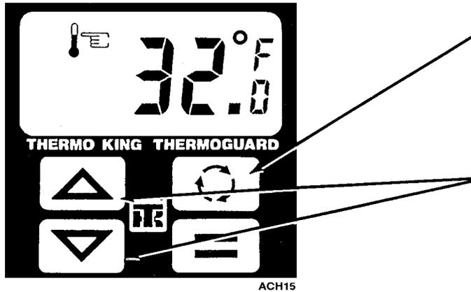
4. Press the SELECT key until the setpoint symbol is again on the screen. However, this time, when the setpoint symbol comes on the screen, DO NOT release the SELECT key, hold it down.
