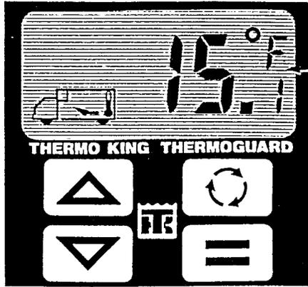
When the Thermo King unit is switched OFF, it is normal for the display to remain on for about 30 seconds as it slowly fades.
