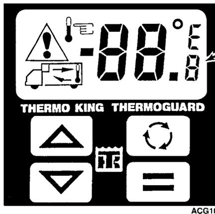
After 5 seconds the standard display will appear. This display remains on the screen during normal operation. The standard display is set to **Return Air Temperature** at the factory, however, the controller can be programmed to show Discharge Air, Return Air, or Setpoint as the standard display.
