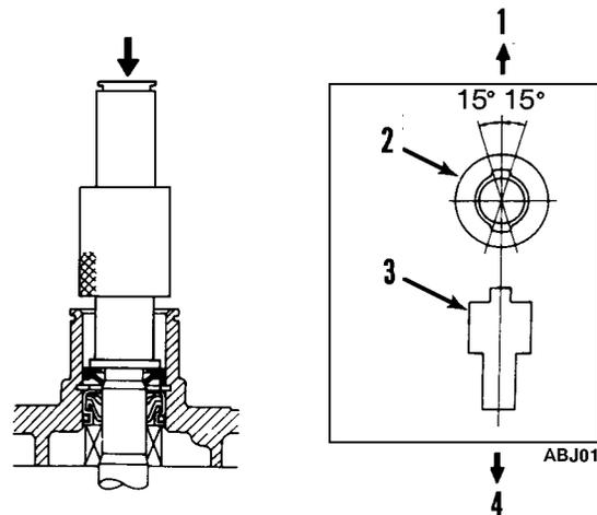
**Proper Shaft Seal Cover Position**
