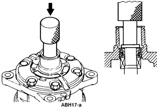
**Press Seal Into Cylinder Head**
