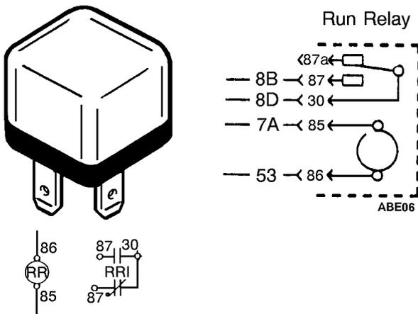
**Relays with Wiring and Schematic
