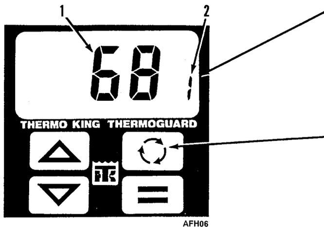
To select other Guarded Access screens, press and release the SELECT key until the desired screen is on the display.
