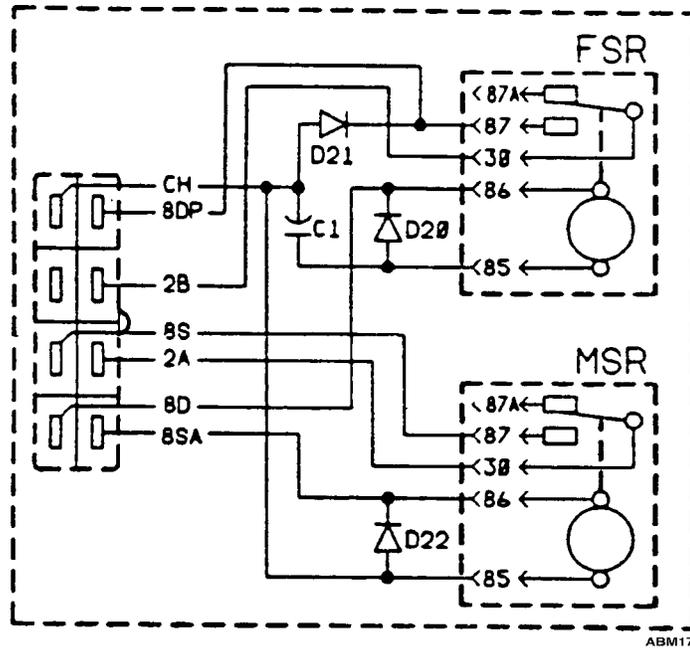
Wiring Diagram of P/N 41-1234 Fuel Solenoid Timer and Manual Start Relay PC Board
