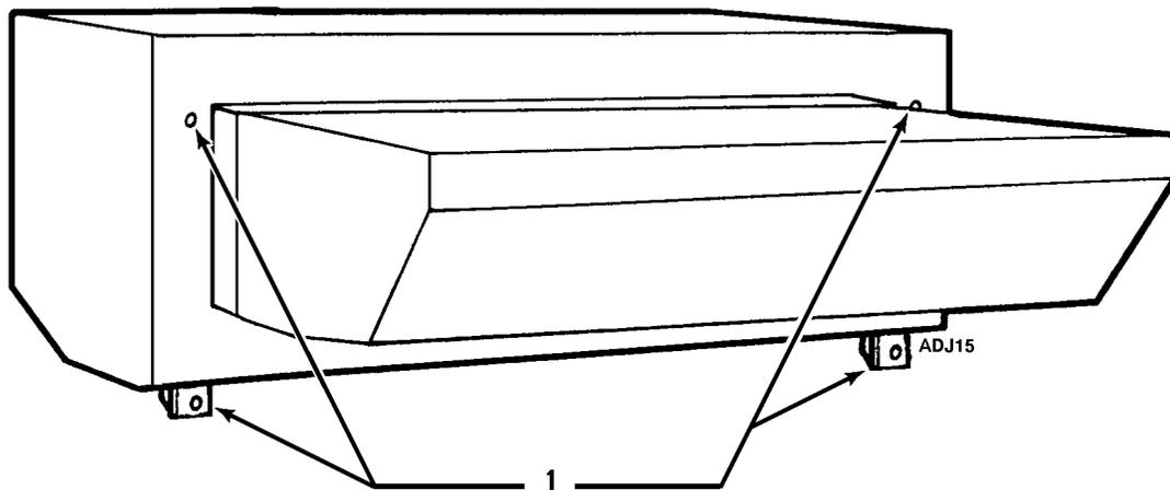
1. Check Mounting Bolts For Tightness
