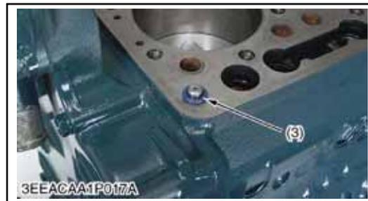
Apply oil to, then re-install the cylinder head bolts.
